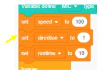
Inserting a negative value (-1) reverses the motor rotation direction.
