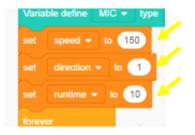
This is where changes can be made in motor speed, motor direction, and/or run time, defined specifically in the three white oval areas (see yellow arrows).
