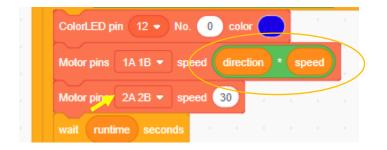
Notice from above (yellow oval) we need to somehow replicate the direction and speed variables in the top Motor block and insert them in the bottom Motor block.
