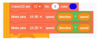
The next and final step is to add and insert the second Motor brake into our script. Notice the Motor brake block location in the mCookie section of mDesigner.
