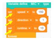
If, we click on the speed value of 150 on set speed, and type in the value of 100 in its place, what do you suppose will happen? If you answered that the motor will turn slower, your answer is correct. Go ahead, change the value to 100 (maximum is 255), upload the altered script into the Windmill and see what happens.
