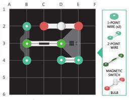
**Step 2:** Place two 1-point wire components one 2-point wire component and the magnetic switch on top of the pieces from step 1, as shown.
