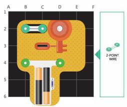
Step 4: Place one 2-point wire component on top of the pieces from step 3, as shown. Put a magnetic over the center opening to make the light go on!
