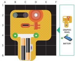
**Step 3:** Add graphic panel and battery. Flip switch on battery to "ON" position.
