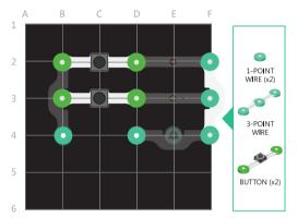
**Step 2:** Place two 1-point wire components, one 3-point wire components and two buttons on top of the pieces from step one, as shown.
