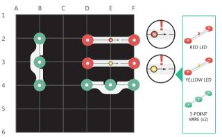
**Step 1:** Place one red LED, one yellow LED, and two 3-point wire components on the board as shown.
