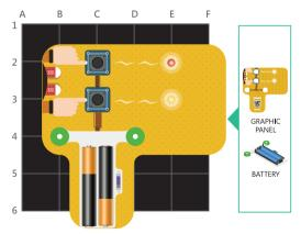
**Step 3:** Add graphic panel and battery. Flip switch on battery to "ON" position.
