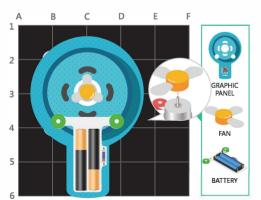
**Step 3:** Add graphic panel, battery, and fan. Flip switch on battery to the "ON" position.
