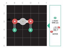
Step 2: Bridge the motor between the two 2-point wire components, and place two 1-point wire components on the board as shown.
