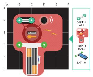
**Step 3:** Place one 2-point wire component on top of the pieces from step 2, as shown. Add graphic panel and battery. Flip switch on battery to the "ON" position.
