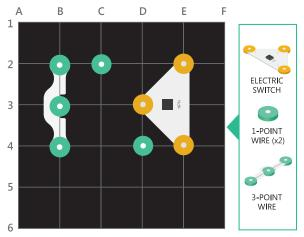
**Step 1:** Place the NPN, two 1-point wire components, and one 3-point wire component on the board as shown.
