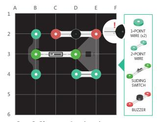
**Step 2:** Place two 1-point wire components, one 2-point wire component, the sliding switch, and the buzzer on top of the pieces from step 1, as shown.
